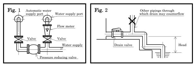
(3) Install the drain piping with an adequate head or inclination as illustrated to insure complete draining. (See Fig. 2.)
